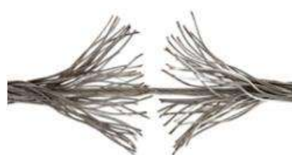
Unraveling of galvanised steel wire
