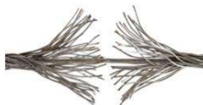
Unraveling of galvanised steel wire
