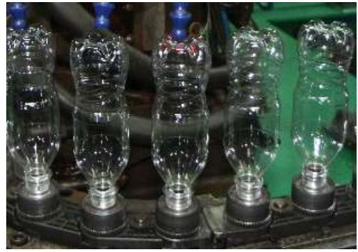
PET bottles after it is blow moulded
