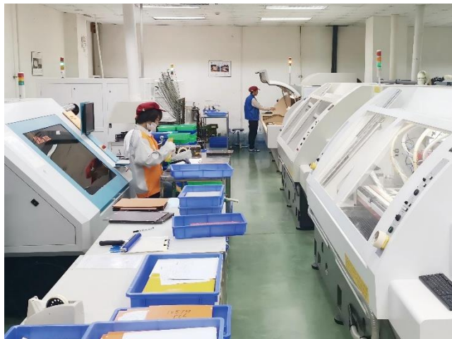
Our CNC drilling
