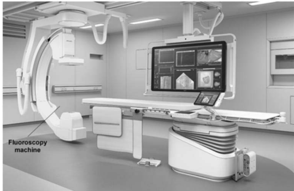
A complete fluoroscopy system incorporating a C-arm fluoroscopy machine
